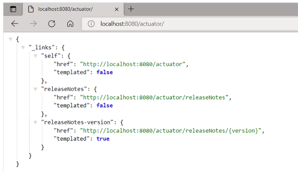
Figure 4.15 Defining custom endpoint /releaseNotes and exposing it through the Actuator discovery page
