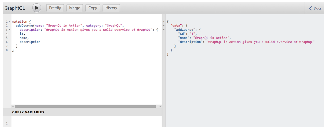
Figure 10.15 Accessing addCourse mutation endpoint to add a new Course. We are accessing the ID, name, and description fields of the newly created course. On the right-hand side, the server presents the requested course details.
